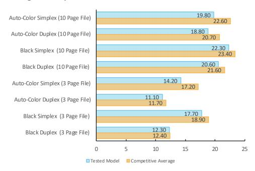
Speed is tested using Buyers Lab's proprietary 3-page and 10-page testing documents. Buyers Lab obtains the overall speed by averaging the tested speed for each run length (1, 5 and 10 sets). The unit was tested using the PCL driver.
