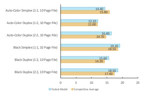
Single-set copy speed is tested using 3-page and 10-page mixed-color and black documents. Timing begins as the start button is pressed, pages are scanned through the document feeder and timing ends when the last page of a single-set of the document exits the device.
