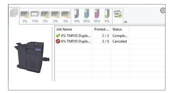
When the user sends a print job a pop up box appears showing all the paper trays and amounts of paper available in each drawer in percent increments, toner remaining in percent increments, and jobs in the print queue. Print job completion and deletion are supported. However, if the user closes out the pop up box during the print process, print job completion and/or deletion will not reappear.
