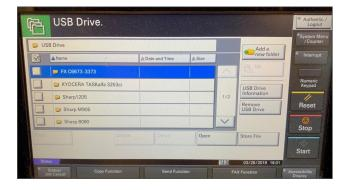
The print from USB menu is automatically populated, with support for PDF, JPEG, and TIFF formats. Users can also change settings for quantity, simplex/duplex, color/mono, and paper size and source. Users can also navigate and print from sub-folders. However, file preview did not function.
